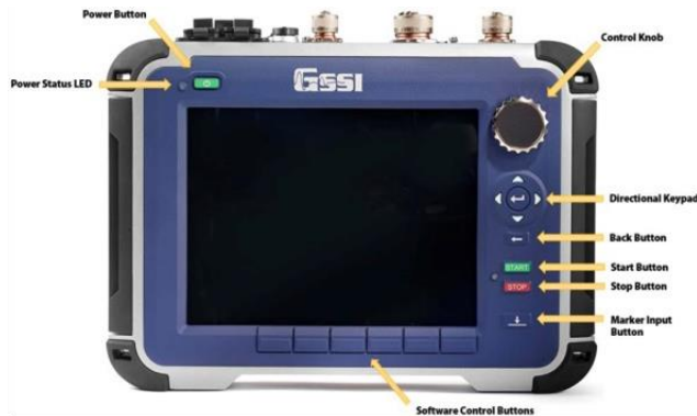
Fig. 3. GPR system used for data collection (SIR 4000 control unit).
