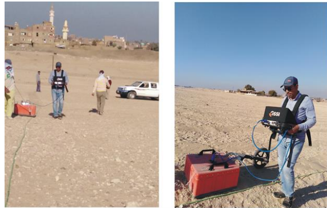
Fig. 4. Photograph of the field acquisition of GPR profiles using the center frequency antenna of 200 MHz.
